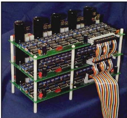
Fig. 5. Gate Driver Boards and MOSFETs for the Multilevel Inverter
