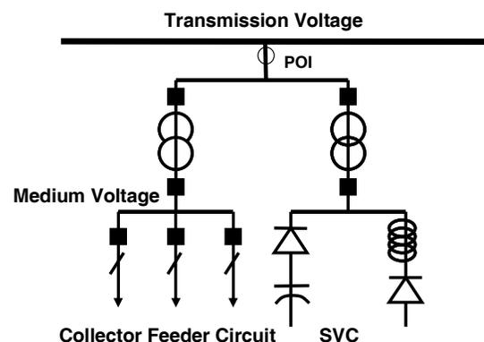
Figure 1. Typical configuration of SVC for WPPs.
