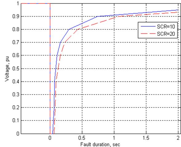
Fig. 3. Voltage ride-through of a wind power plant with induction machines without any additional ride-through measures as a function of the short circuit ratio.
