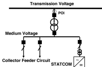
Figure 2. Typical configuration of STATCOM for WPPs.
