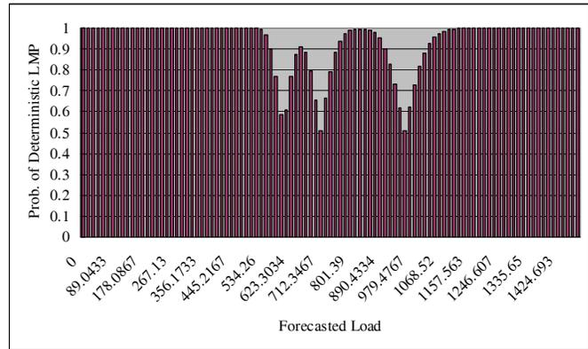
Fig. 7. Probability of deterministic LMP at bus B versus forecasted load (with 10% price tolerance).
