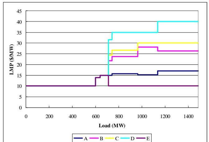
Fig. 1. LMP at all buses with respect to different system loads for the modified PJM 5-bus system.
