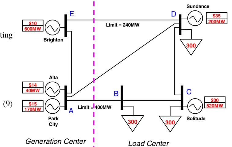
Fig. 5. The Base Case Modified from the PJM Five-Bus Example.
