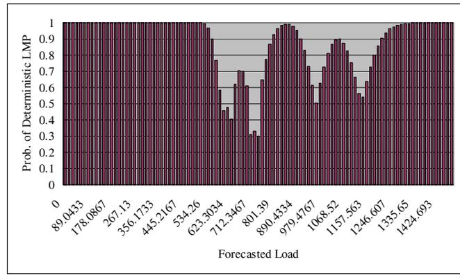
Fig. 6. Probability of deterministic LMP at bus B versus forecasted load.
